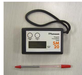
Photo 1 SM20 type portable susceptibility indicator made by ZH Instruments.
